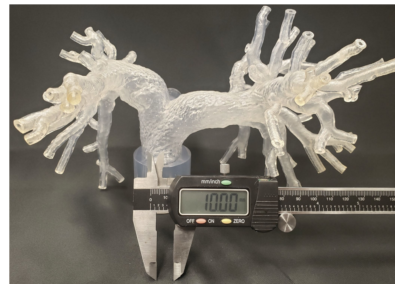
3D printed patient-specific phantom
