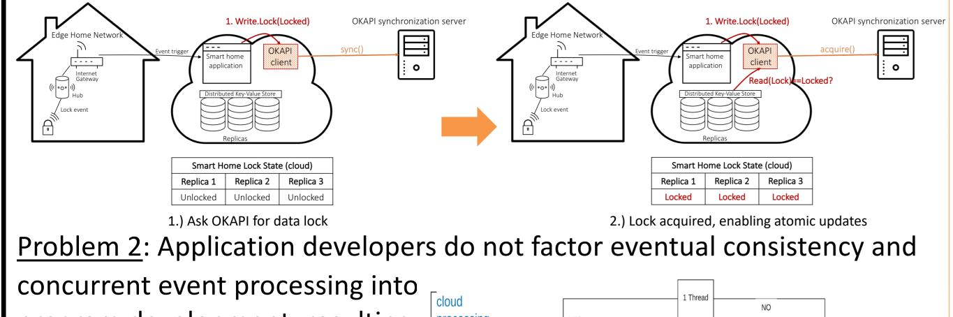
concurrent event processing into program development, resulting in incorrect applications. **Approach**: Create static analysis tools to identify application code that may result in lost updates or reordered updates to cloud and device state.
