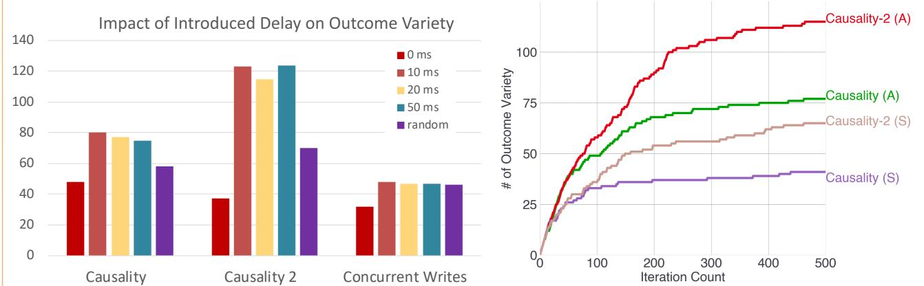
Demonstrating the variability of outcome variety obtained through Musli Tool based on data update delay (left) and RPC Request type (right: synchronous (S), asynchronous (A)).
