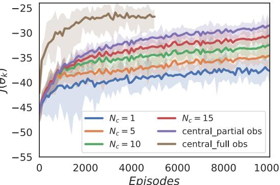
The performance of the proposed distributed RL algorithm gets closer to that of the centralized algorithm under partial observation scenario as  $N_c$  increases .
