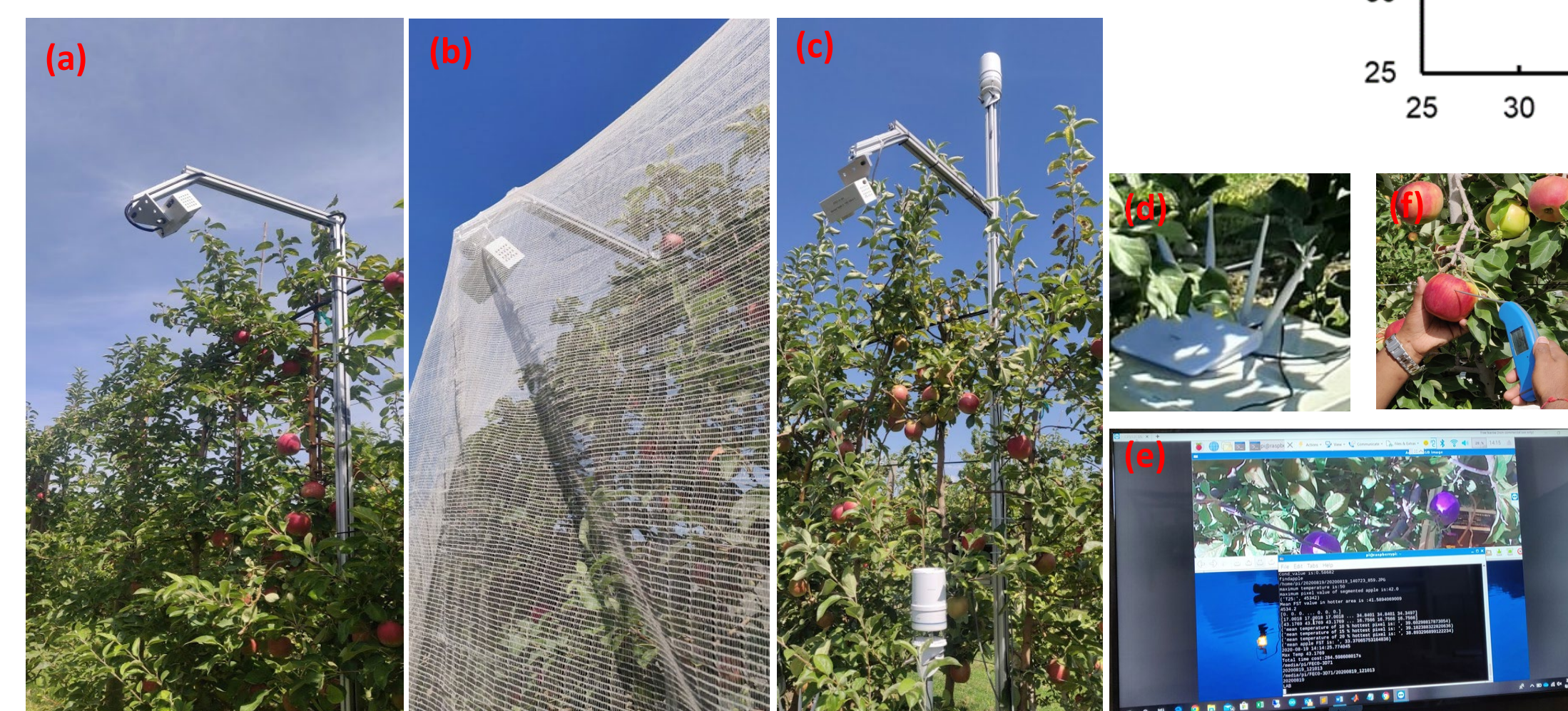
Fig. 2. CPSS2.0 node deployed in (a) wet zone of modified evaporative cooling, (b) shade net, and (c) untreated control with two all-in-one weather sensors within and above the canopy to monitor imagery and weather-based fruit surface temperature and (d) in-field cellular router to create a local WiFi grid to add connectivity and (e) remote data access; (f) FST ground truthing
