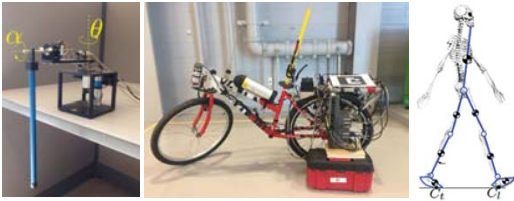
Figure 1: A set of example of human cyber-physical balance systems, such as Furuta pendulum, autonomous bikebot and bipedal walkers (from left to right).
