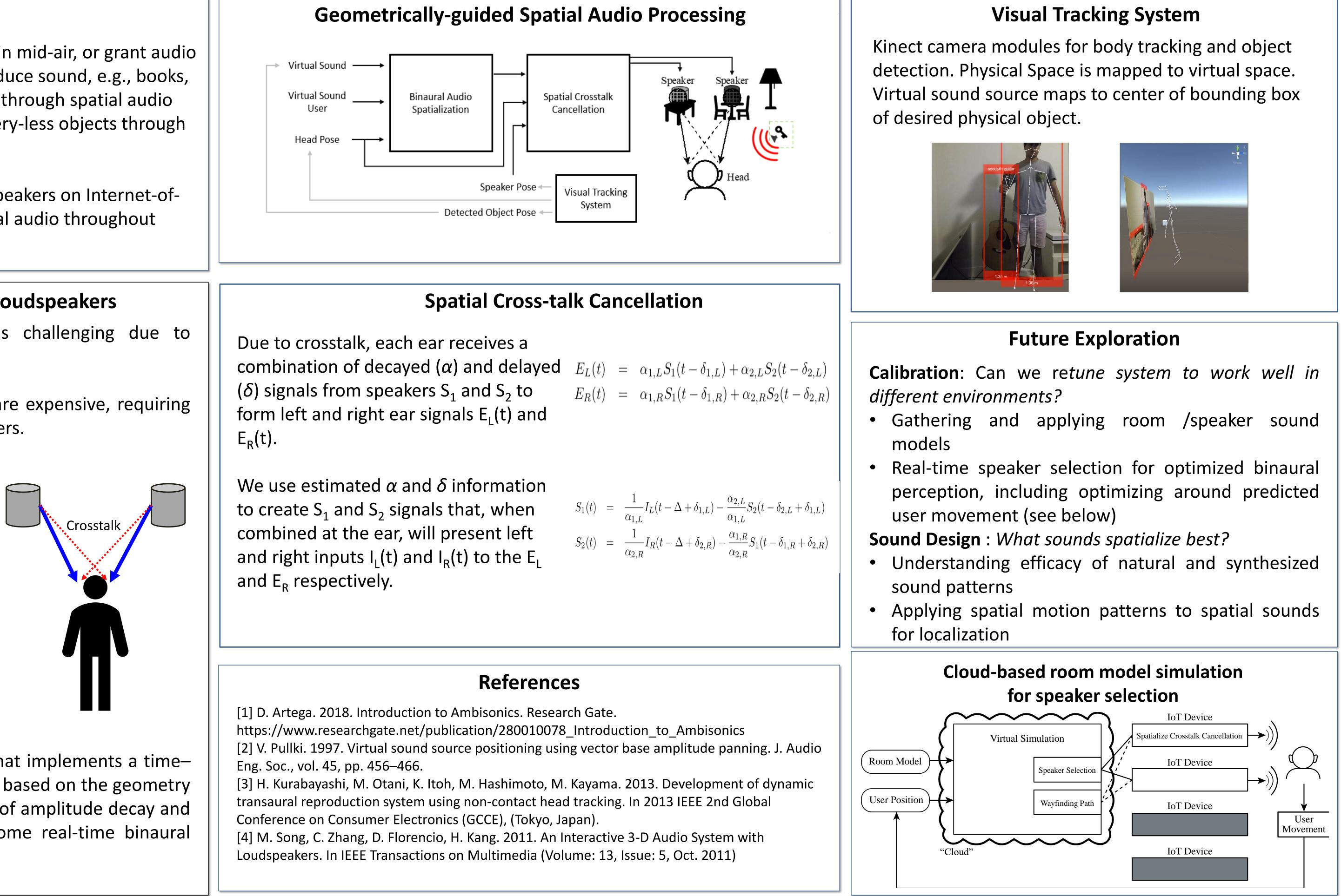
We propose a distributed spatial audio system that implements a timedomain dynamic crosstalk cancellation technique based on the geometry of a user's head position which uses estimations of amplitude decay and time delay to produce sound signals that become real-time binaural audio at the user's ears.
