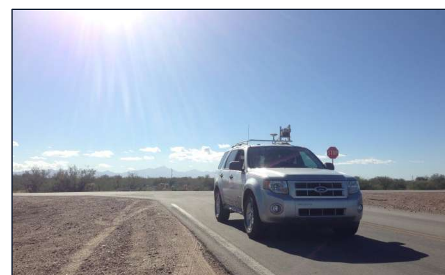
The CAT Vehicle with SICK laser scanner mounted on the roof.
