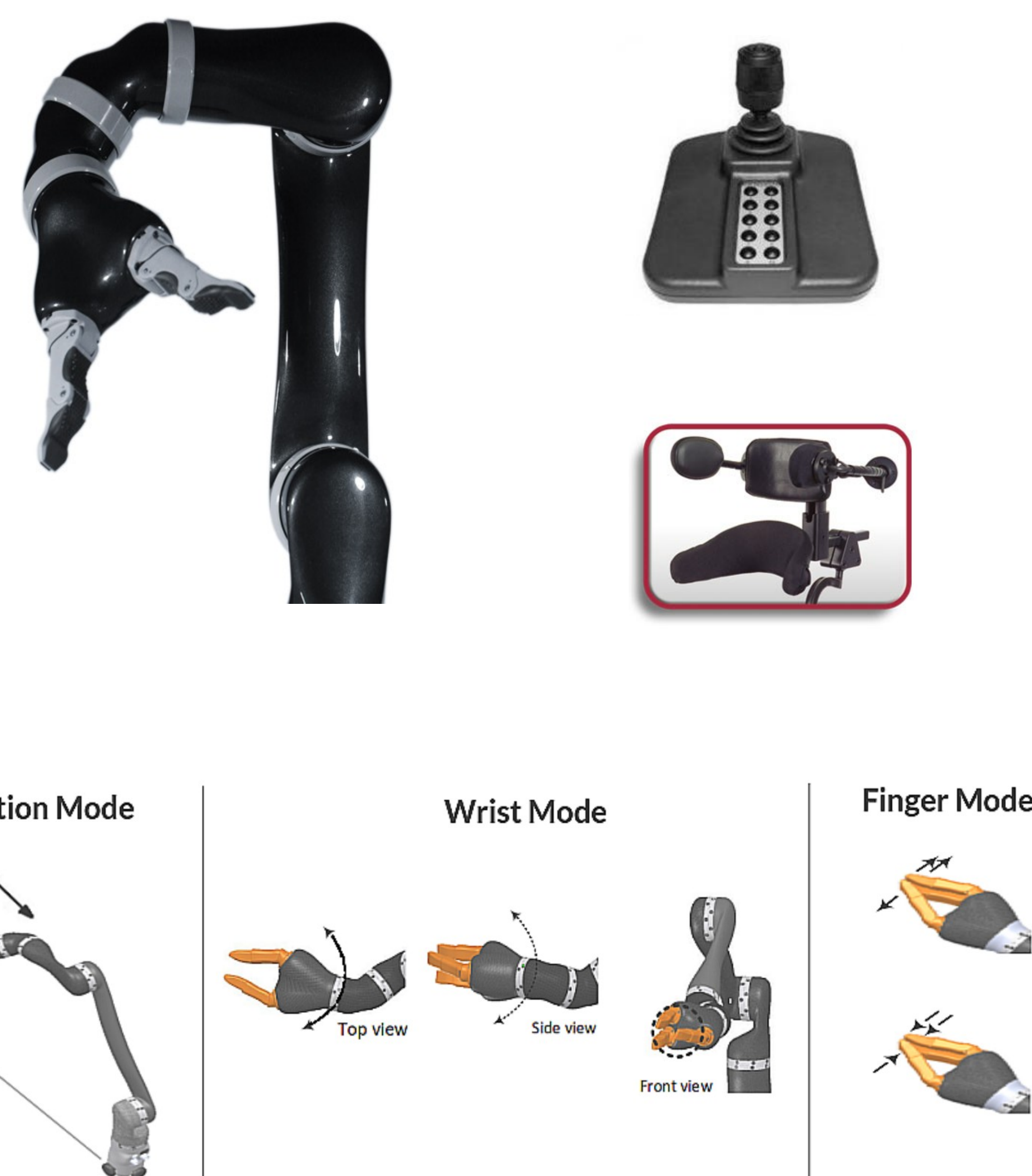
Figure 1: 7DoF robotic arm. Control interfaces: 2D joystick and 1D head array (Top). An example of partitioning of 7D control space to form control modes for operating the robotic arm (Bottom).
