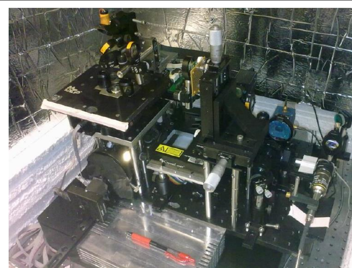
Custom made optical tweezer setup, used in PI's Nanodynamics lab at the University of Minnesota, Twin Cities
