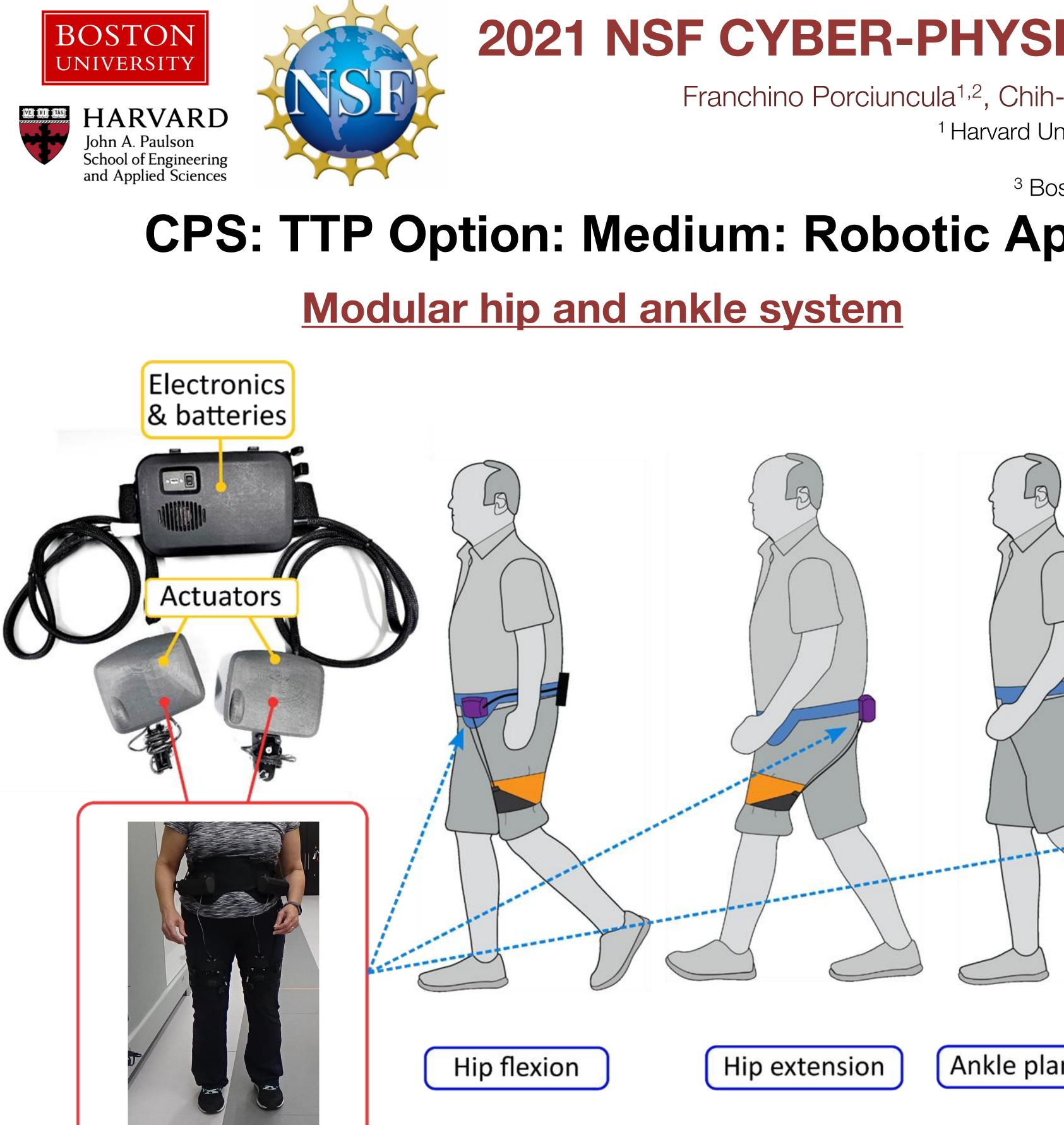
Modular actuator design allows to place the actuators at different target joints depending on the purpose and the user population • New small and lightweight actuator using a miniature rope winch
