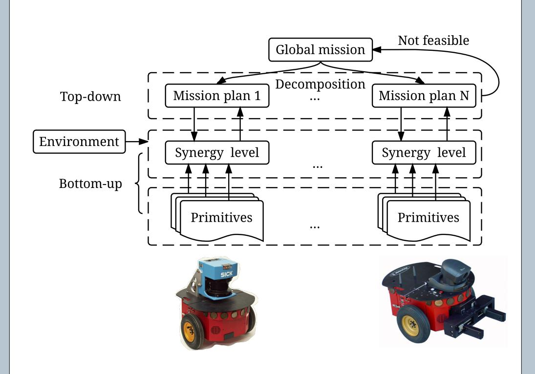
We propose to **combine** top-down and bottom-up approaches so to com up with a scalable formal **correct-by-design** method for distributed coordination and control of multi-robot systems in **uncertain** environments.
