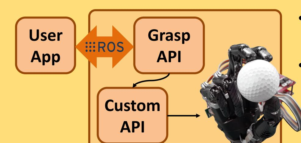
Custom programming interface for a commercial robotic prosthetic hand using a high-level ROS wrapper on top of the low-level API to allow selection of parameterized grasp types.
