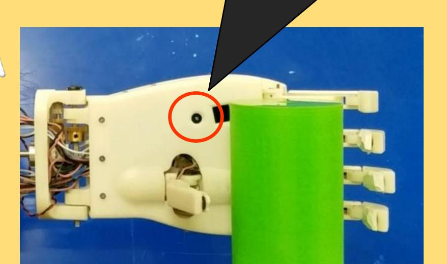
A touch button positioned at wrist is used to initiate grasping a cube object.
