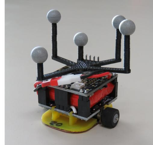
The Robotarium's main inhabitant: the GRITSbot is a small, differential-drive robot equipped with:
