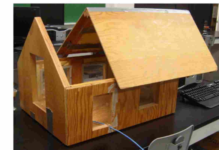
"Little House in Alaska" building heat flow model
