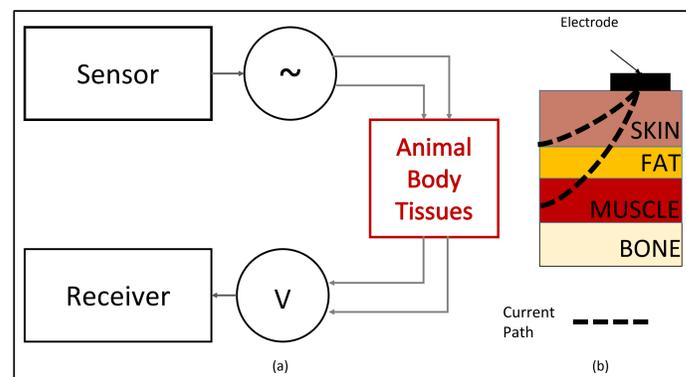
**Galvanic Coupling:** (a) Basic Circuit layout and (b) Dissipation of current through the layers of body tissues.
