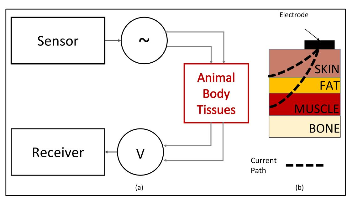
Galvanic Coupling: (a) Basic Circuit layout and (b) Dissipation of current through the layers of body tissues.
