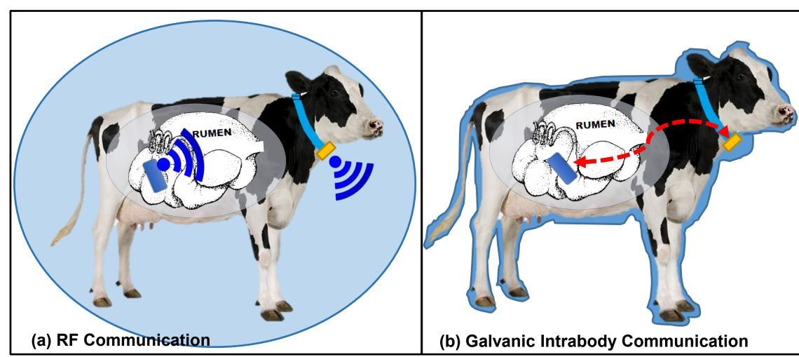
Comparison of the field radius of RF and Intrabody Communication.
