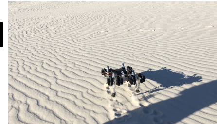
Minitaur: rapidly “scouting” spatial variation of soil erodibility
