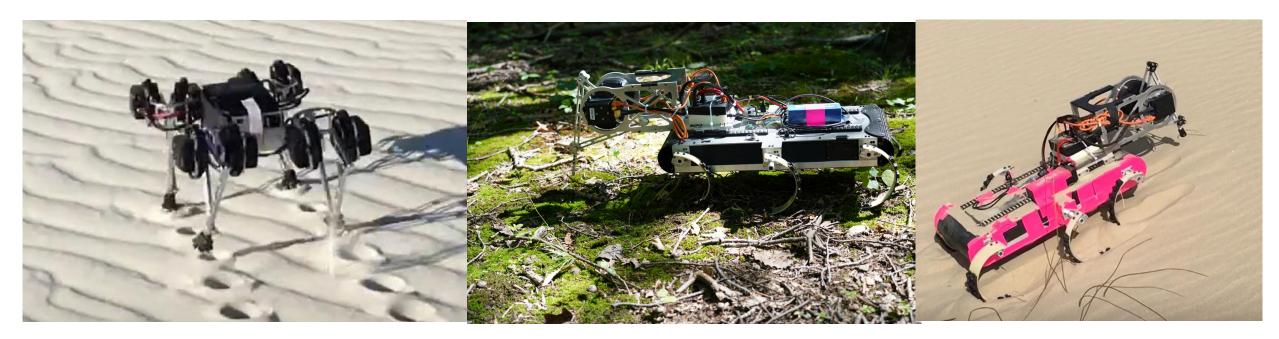
We develop novel geoscientific instrumentation embodied in robots' legs, and deploy the robots at White Sands, NM, Oceano, CA, and Wissahickon, PA to characterize the mechanical properties of soil that determine its resistance to erosion and transport by overland flow and creep. Such information is critical in understanding sediment loss to wind and rivers, and provides insights on soil stability in landslides and desertification processes.
