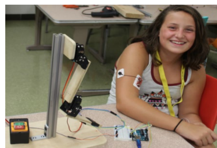
Student uses muscle signals to control Neu-pulator
