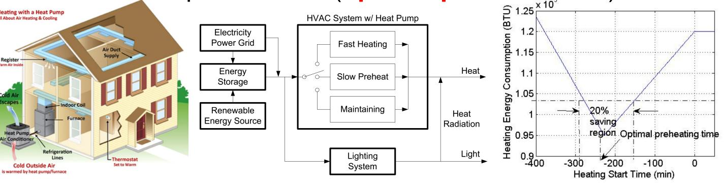
Observation: 54% energy saving under optimal preheat strategy; At least 20% saving as long as in 1-hour window containing optimal preheat time
