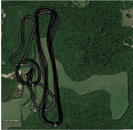
Fig.1. GPS trajectory of KHawk UAS flight 1.
