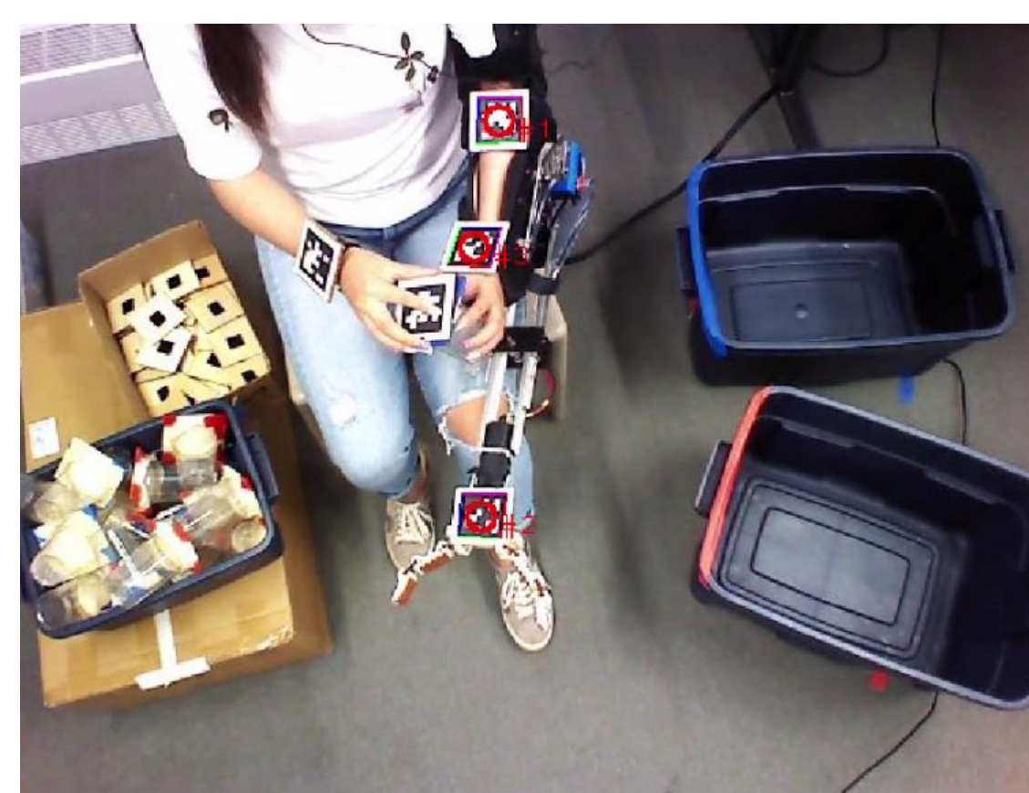
View from stereo camera used for tracking the cups, human poses and robot poses,
