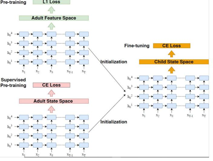
Illustration of supervised and unsupervised pre-training (transfer learning). The blue parts are the LSTM layers to be transferred.
