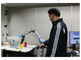
We create effective direct control interfaces by mapping from the user's movements to robot actions. [HRI17] The mapping must preserve the feasibility of the robot motion while approximating the input movement. We provide such mappings in a solver called RelaxedIK [RSS18].
