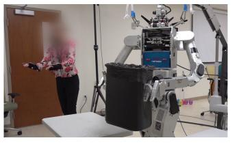
[SciR19] allowing a user to control a pair of robot arms. To provide an effective interface, the system infers appropriate assistance modes based on the movements. Recent work also considers the effects of latency and robot speed on task performance [HRI20b]
