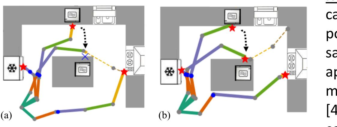
Above: Algorithm results show coverage differences between two designs in a simulated kitchen environment. (a) Without a coverage function, if the microwave is moved from the counter to the island, it is no longer a reachable target. (b) With the addition of the coverage function, the design has a greater coverage and can still reach the microwave even if it is moved. The algorithm can also find different sequences of reaching the four targets.
