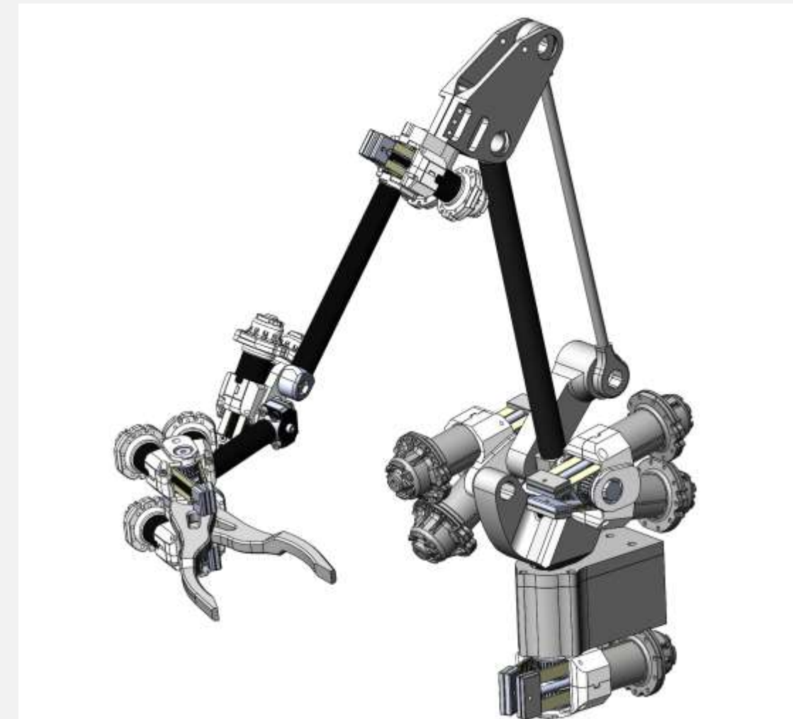
Under devel. 7-DOF arm, fully remotely actuated
