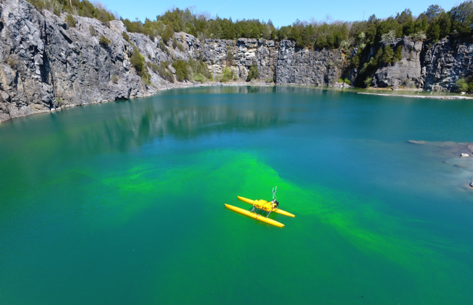
USV sampling of fluoroscein plume
