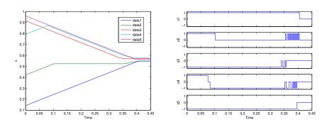
Sample evolutions of states x and corresponding controls u on a ring with n=5 nodes,  $\varepsilon=0.02$
