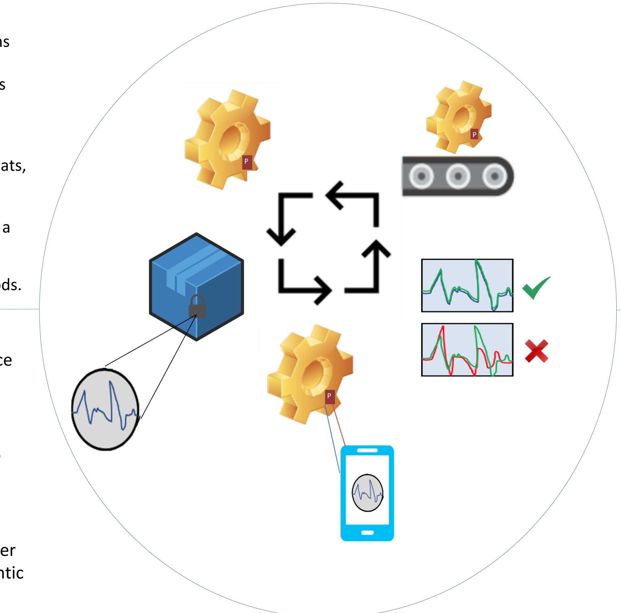
Tracking a component throughout a supply network: the physical measurement uniquely identifies the part and is asserted to match a ground truth identity until the part reaches the intended consumer.
