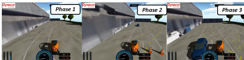
Figure 36: Example of the double lane change maneuvers in three phases, with Dynacac
