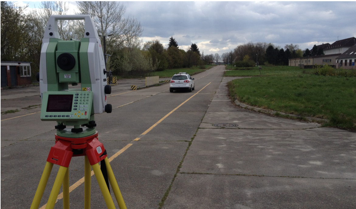
Figure 3: Final setup on 2016/04/19 for execution of testdrives: Tracking tachymeter placed directly behind vehicle for better visibility of marker on vehicle. FASCAR2 facing down reference track (north-to-south) at Heinrich-Der-Löwe-Kaserne, Braunschweig.
