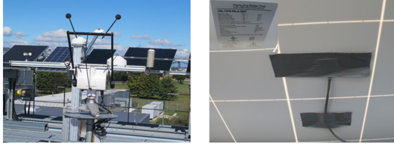
Figure 17: Weather station (on the left) and module temperature sensor (on the right).
