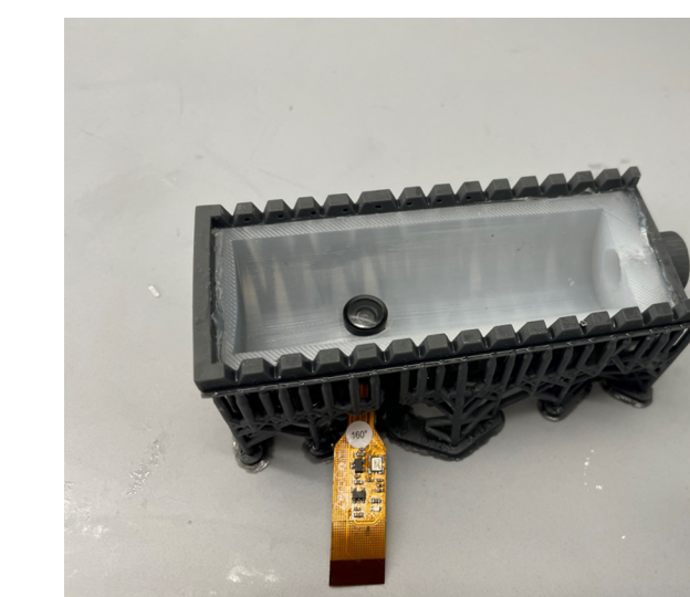
Embedded camera to observe the contact surface
