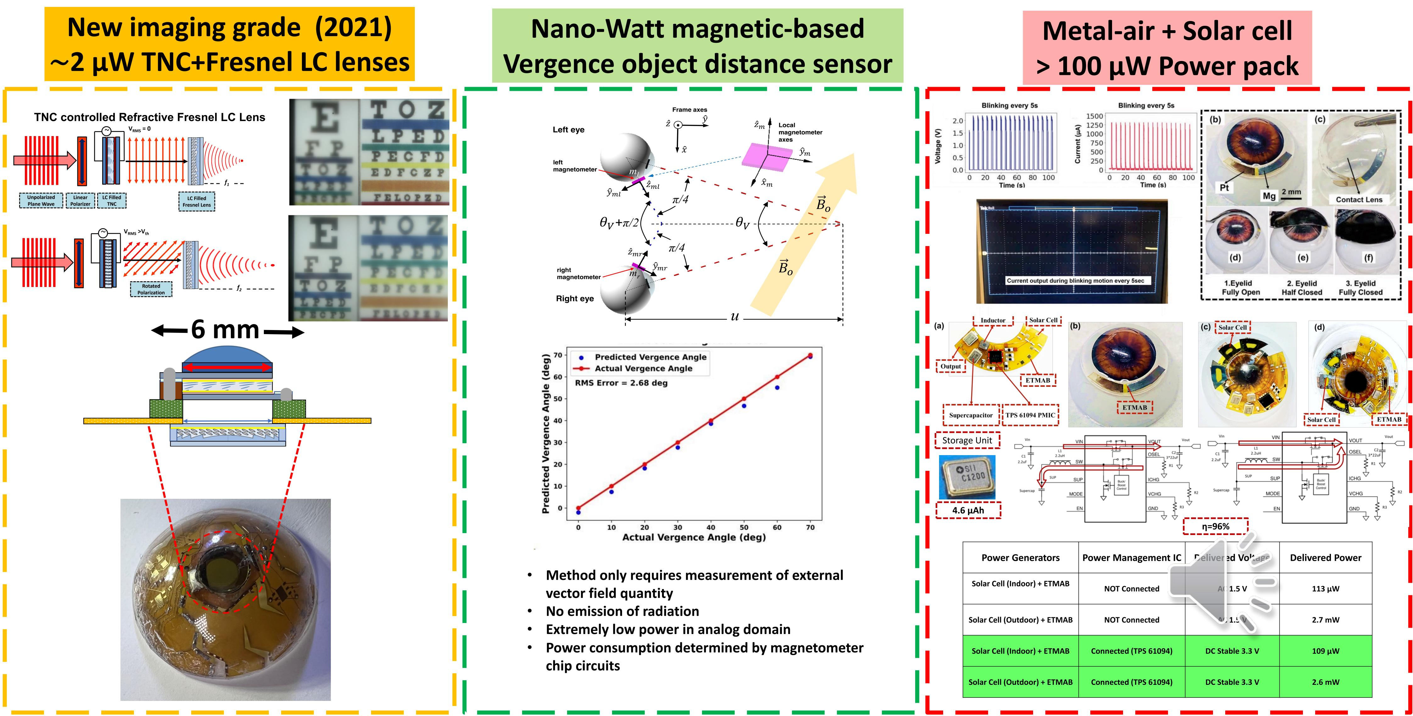
Developed imaging grade 2-µW Twisted Nematic Cell -based varifocal liquid crystal lens Developed nano-Watt magnetic-based object range finder Developed eyelid motion Mg-Air battery + solar cells Integrated power pack > 100  $\mu$ W sustained Developed low-power PWM algorithms for controlling tunable lens
