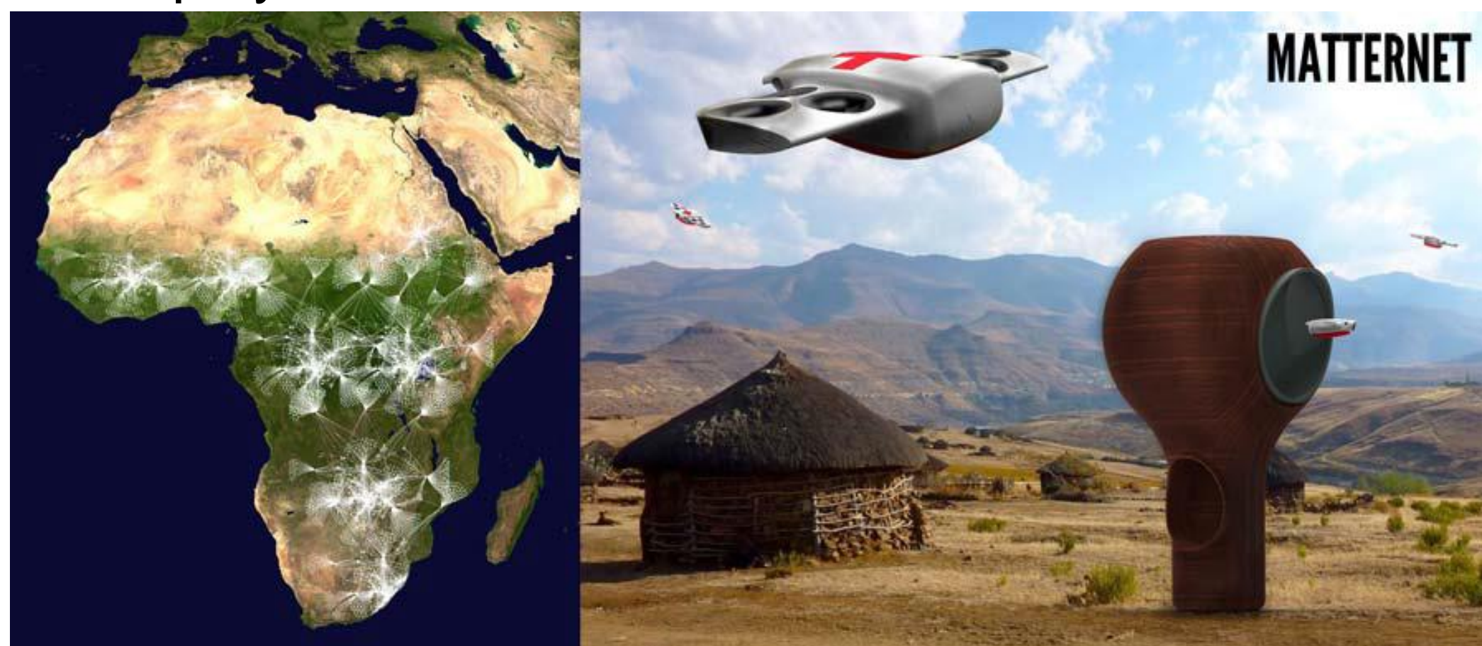
Fig. 1. Matternet envisions a team of small UAVs that can form a network to deliver much needed medicine in Africa. UAV network (left) and Matternet UAVs (right) are shown.
