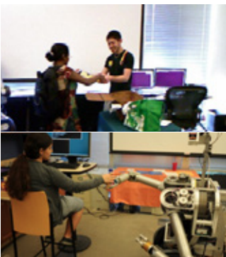
People handed over objects to the above robot more efficiently when it utilized human physical collaboration cues.
