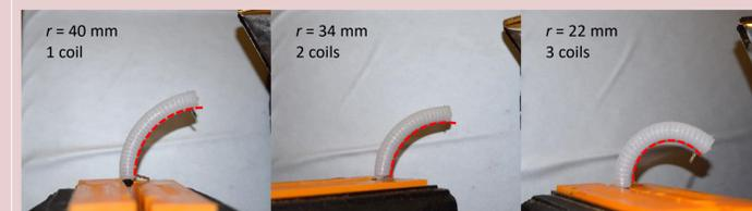
Combined pressurization of the cavity and contraction of the SMA coils results in an apparent increase in stiffness of the actuator.
