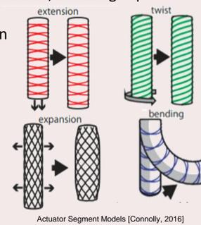
Similar to examples seen in nature such as a Venus flytrap plant and the muscular hydrostats, here the combination of hydrostatic pressure and constraints imposed by inextensible fibers creates unique bending behavior.
