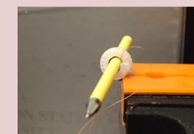
The bending of the PneuSMA actuator is described using a simplified modeling approach based on the linear stiffness of the silicone rubber and finite element analysis of parallel springs along the length of the actuator. This model accounts for the lengthening of the actuator due to the pressure on the inside walls of the actuator, the spring force from the SMA coils, and the effective spring forces from the silicone material.
