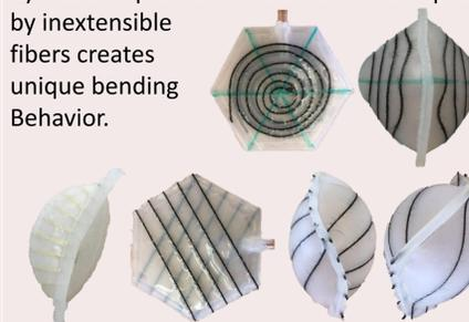
Experimental measurements of a simple bending module are shown on the right. Developing a model to describe the bending and twisting behavior of the different modules and combinations of multiple units will be the focus of future work.
