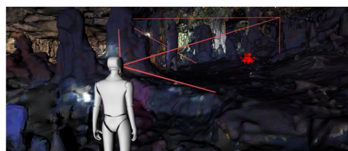
Figure 2: Applying a spatial constraint (i.e., helmet mounted camera) to the exploration objective reduces uncertainty in shared human-robot map [1].
