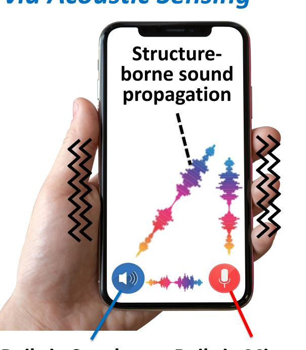
Structure-borne sound propagation depends on materials, dimensions, and external forces of the device and the user's hand
