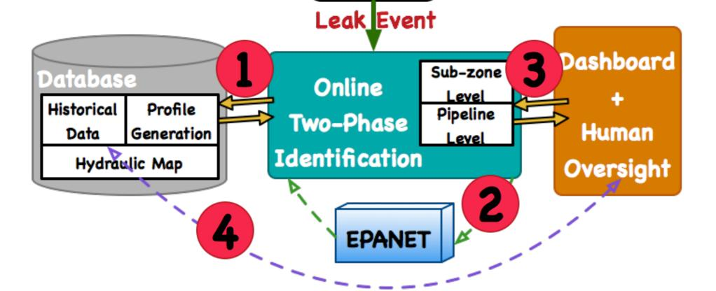
4. Trigger corresponding adaptations (e.g. actuation and control of water infrastructure elements). Update database to refine sensor selection and placement, pipeline distribution and replacement etc.
