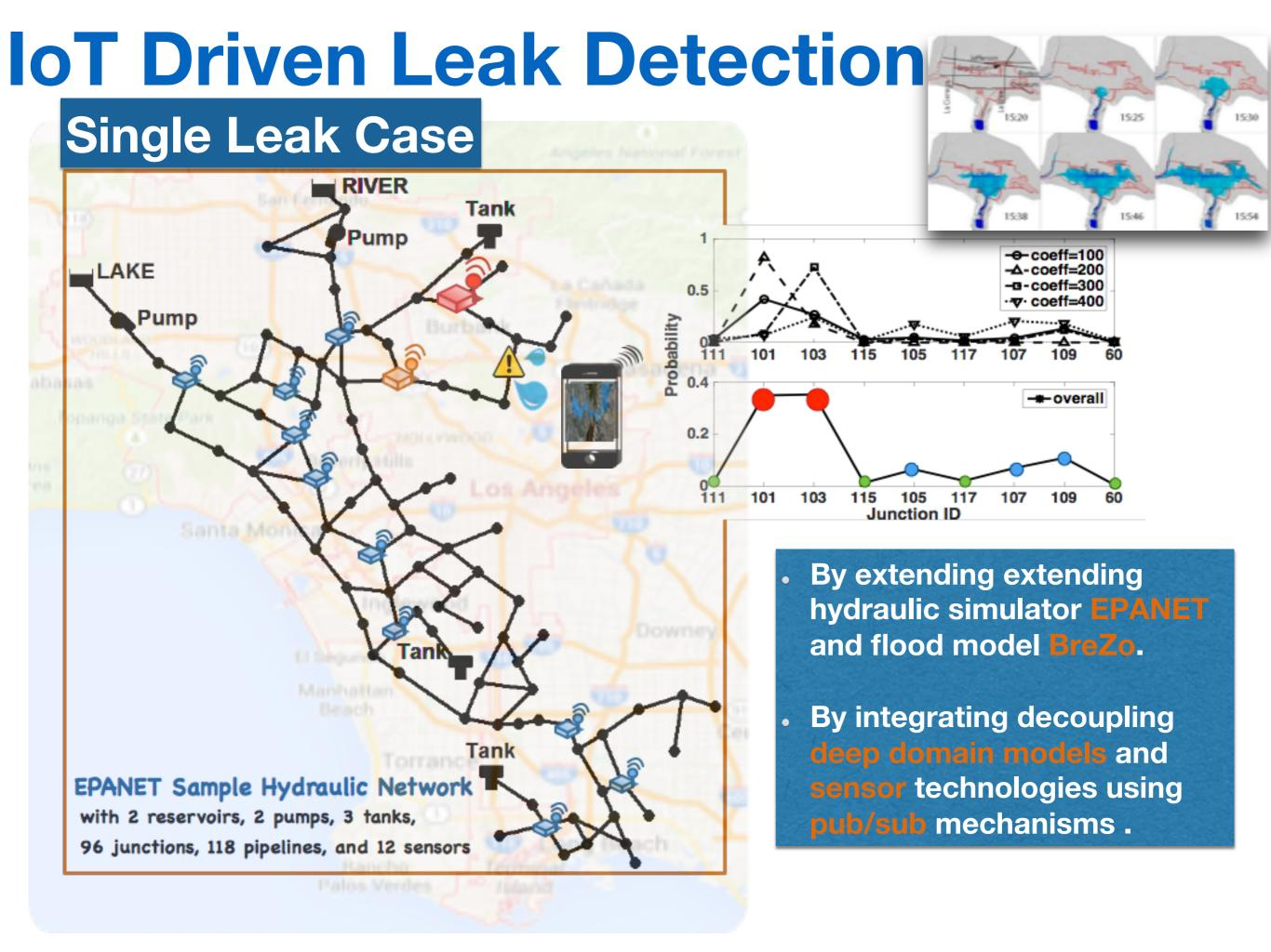
**IoT Driven Leak Detection**
