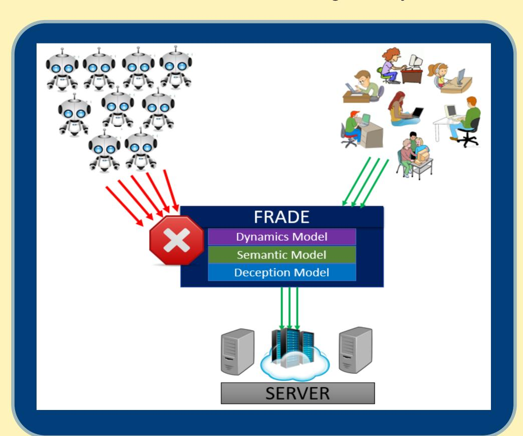
FRADE models three different aspects of human interaction with application-level content to distinguish humans from bots: request dynamics, request semantics and how humans process visual cues. While bots can trick FRADE's models, they must severely reduce their request output. This forces attackers to use orders-of-magnitude larger botnets for a successful attack.
