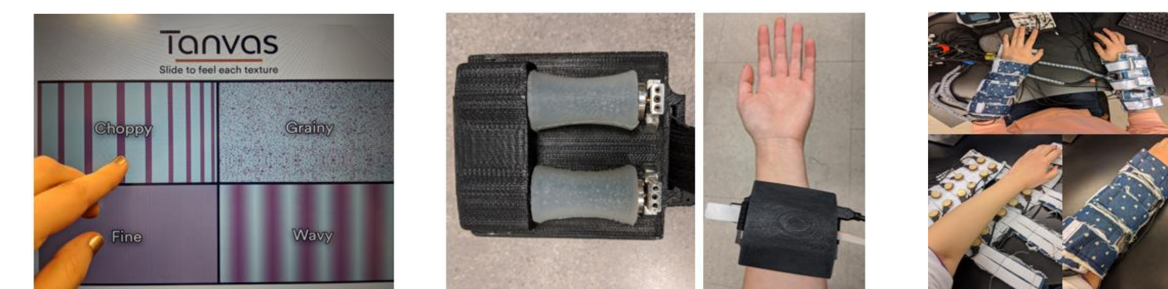
Mimo Vue Monitor With Tanvas Touch Friction Display. The Surface Haptics Enable Friction Modulation To Convey Texture Information.
