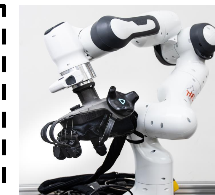
Upper-limb haptic interface Panda robotic arm with HaptX glove
