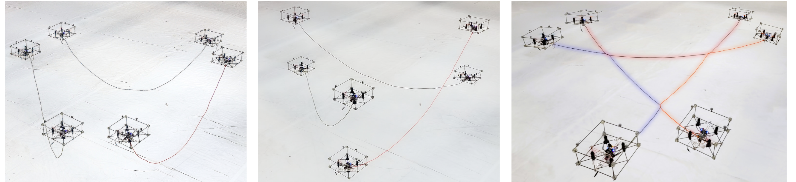
(a) Step 1: Free catenary robots [1] (b) Step 2: Interlacing cables (c) Step 3: Triangular hitch Figure: Action 1: Six quadrotors forming a triangular polygonal hitch.
