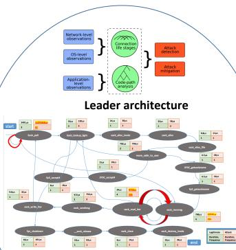
Connection life diagram showing differences in legitimate and attack connections
