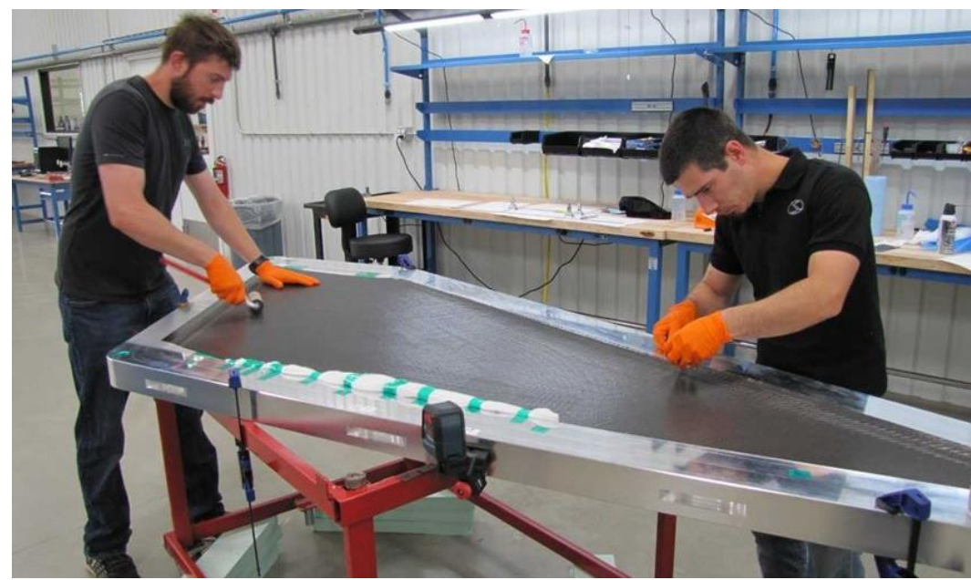
Ongoing Layup (Source: Modernmachineshop 2018)
