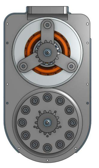
D Powered, Backdrivable Ankle Joints have been developed to facilitate standing and walking balance. While stimulated muscle is still used for propulsion, it lacks the bandwidth and controllability for fine control work. These robotic actuators have the required response time and bandwidth for balance control.
