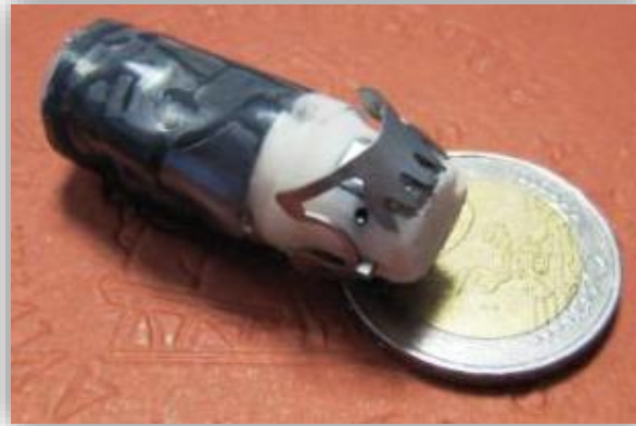
Clip releasing capsule, Valdastri et al., 2008
