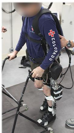
**LEFT:** Individual with thoracic level SCI with implanted stimulating electrodes stands and walks while wearing the CPWS. In this walking experiment, the pilot's muscles are controlled by a typical walking pattern while ballistic control at the motors assists with completing the movement.
