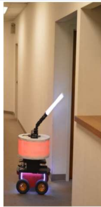
Previously built evacuation robot in research by Robinette, Howard, and Wagner
