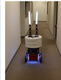
Previously built evacuation robot in research by Robinette, Howard, and Wagner
