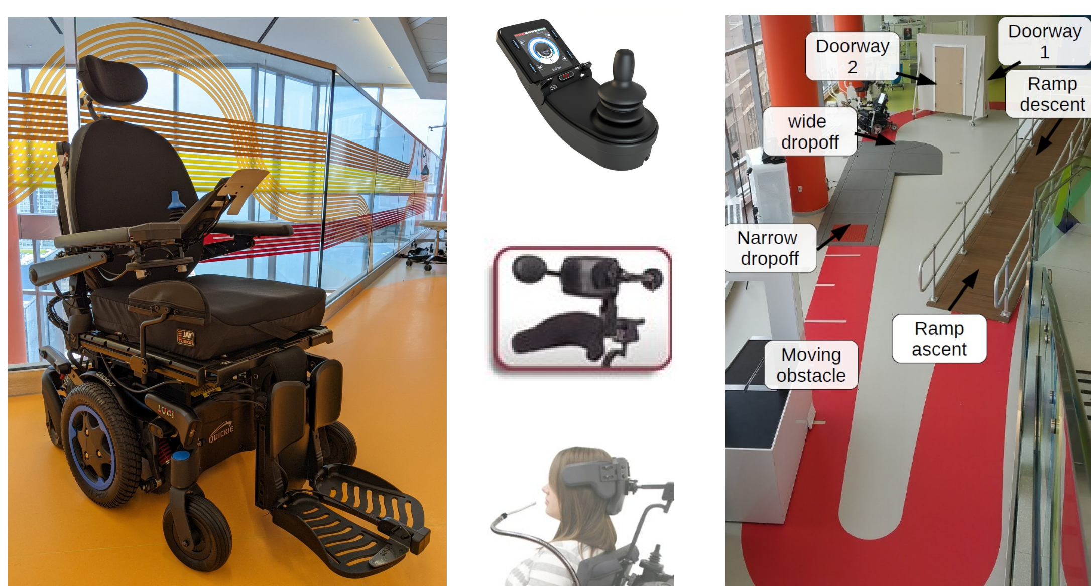
Figure 2: Application domain: human operators with motor impairments. Shared-control robotic wheelchair and control interfaces (2-axis joystick, switch-based head array, sip-and-puff), differ in activation , dimensionality , and proportionality .
