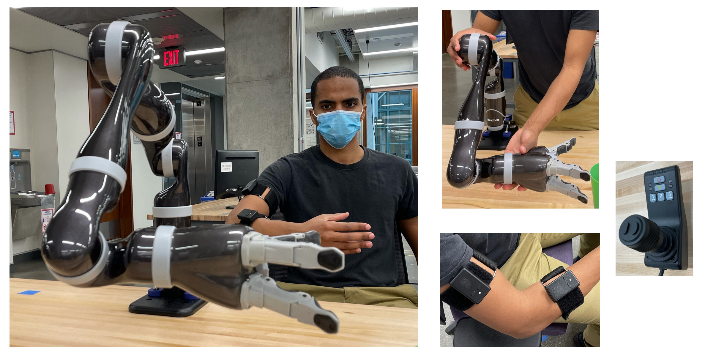
Figure 3: Application domain: Robot learning from human instructors. Robotic arm and control interfaces (3-axis joystick, motion tracking via IMUs, kinesthetic operation), differ in activation , dimensionality , and proportionality .
